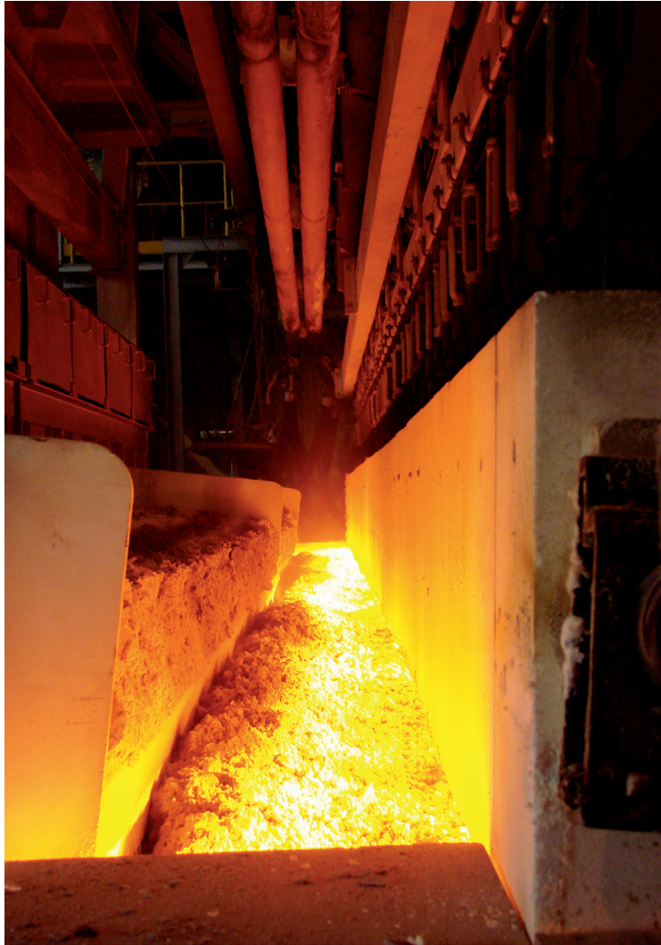
Raw Material added to the oil fired furnace Glas Trösch Flat Glass Plant
