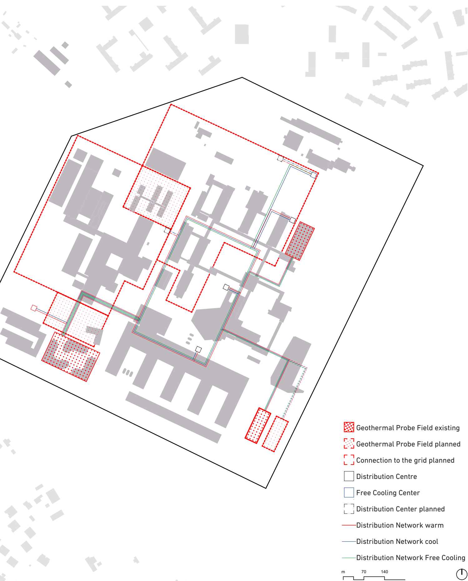
berg with the associated geothermal probe fields, pipe-networks and distribution centres
